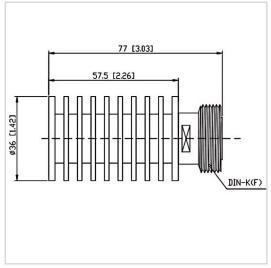
RF Solution offer a wide selection of Coaxial Fixed Termination (Dummy Load) for global customers. CT-20W-RA3657-DINK-4G is Coaxial Termination (Dummy Load) in Frequency Range of DC~4.0 GHz. It is made of high quality materials under a high standard, the Connector Type of this product is DIN-F (K), VSWR Max is 1.20 and Impedance is 50  $\Omega$ . The component has a good working performance and stability, it is ideal for handling a Power of 20 W.
