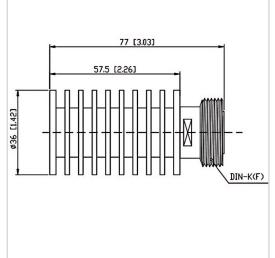
RF Solution offer a wide selection of Coaxial Fixed Termination (Dummy Load) for global customers. CT-20W-RA3657-DINK-3G is a Coaxial Fixed Termination (Dummy Load) in Frequency Range of DC~3.0 GHz. It is made of high quality materials under a high standard, the Connector Type of this product is DIN-F (K), VSWR Max is 1.20 and Impedance is 50  $\Omega$ . The component has a good working performance and stability, it is ideal for handling a Power of 20 W.
