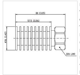
RF Solution offer a wide selection of Coaxial Fixed Termination (Dummy Load) for global customers. CT-20W-RA3657-DINJ-4G is a Coaxial Fixed Termination (Dummy Load) in Frequency Range of DC~4.0 GHz. It is made of high quality materials under a high standard, the Connector Type of this product is DIN-M (J), VSWR Max is 1.25 and Impedance is 50  $\Omega$ . The component has a good working performance and stability, it is ideal for handling a Power of 20 W.
