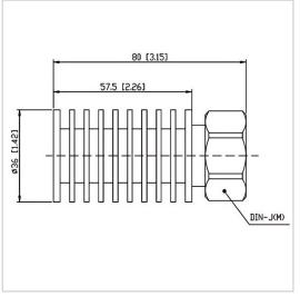
RF Solution offer a wide selection of Coaxial Fixed Termination (Dummy Load) for global customers. CT-20W-RA3657-DINJ-3G is а Coaxial Termination (Dummy Load) in Frequency Range of DC~3.0 GHz. It is made of high quality materials under a high standard, the Connector Type of this product is DIN-M (J), VSWR Max is 1.20 and Impedance is 50  $\Omega$ . The component has a good working performance and stability, it is ideal for handling a Power of 20 W.
