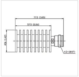
RF Solution offer a wide selection of Coaxial Fixed Termination (Dummy Load) for global customers. CT-20W-RA3657-4310K-6G is a Coaxial Termination (Dummy Load) in Frequency Range of DC~6.0 GHz. It is made of high quality materials under a high standard, the Connector Type of this product is 4.3-10-F (K), VSWR Max is 1.30 and Impedance is 50  $\Omega$ . The component has a good working performance and stability, it is ideal for handling a Power of 20 W.
