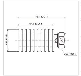
RF Solution offer a wide selection of Coaxial Fixed Termination (Dummy Load) for global customers. CT-20W-RA3657-4310J-6G is a Coaxial Fixed Termination (Dummy Load) in Frequency Range of DC~6.0 GHz. It is made of high quality materials under a high standard, the Connector Type of this product is 4.3-10-M (J), VSWR Max is 1.30 and Impedance is 50  $\Omega$ . The component has a good working performance and stability, it is ideal for handling a Power of 20 W.
