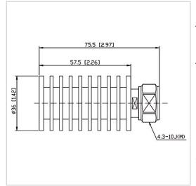
RF Solution offer a wide selection of Coaxial Fixed Termination (Dummy Load) for global customers. CT-20W-RA3657-4310J-4G is a Coaxial Fixed Termination (Dummy Load) in Frequency Range of DC~4.0 GHz. It is made of high quality materials under a high standard, the Connector Type of this product is 4.3-10-M (J), VSWR Max is 1.30 and Impedance is 50  $\Omega$ . The component has a good working performance and stability, it is ideal for handling a Power of 20 W.
