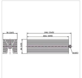
RF Solution offer a wide selection of Coaxial Fixed Termination (Dummy Load) for global customers. CT-200W-FA8022-NK-6G is a Coaxial Fixed Termination (Dummy Load) in Frequency Range of DC~6.0 GHz. It is made of high quality materials under a high standard, the Connector Type of this product is N-F (K), VSWR Max is 1.30 and Impedance is 50  $\Omega$ . The component has a good working performance and stability, it is ideal for handling a Power of 200 W.
