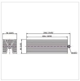
RF Solution offer a wide selection of Coaxial Fixed Termination (Dummy Load) for global customers. CT-200W-FA8022-NK-4G is Coaxial а Termination (Dummy Load) in Frequency Range of DC~4.0 GHz. It is made of high quality materials under a high standard, the Connector Type of this product is N-F (K), VSWR Max is 1.30 and Impedance is 50  $\Omega$ . The component has a good working performance and stability, it is ideal for handling a Power of 200 W.
