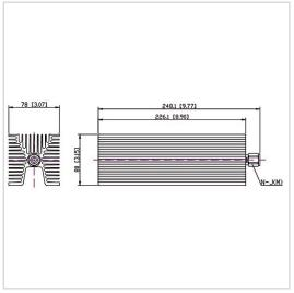
RF Solution offer a wide selection of Coaxial Fixed Termination (Dummy Load) for global customers. CT-200W-FA8022-NJ-6G is a Coaxial Fixed Termination (Dummy Load) in Frequency Range of DC $\sim$ 6.0 GHz. It is made of high quality materials under a high standard, the Connector Type of this product is N-M (J), VSWR Max is 1.30 and Impedance is 50  $\Omega$ . The component has a good working performance and stability, it is ideal for handling a Power of 200 W.
