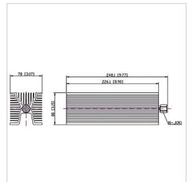
RF Solution offer a wide selection of Coaxial Fixed Termination (Dummy Load) for global customers. CT-200W-FA8022-NJ-4G is a Coaxial Fixed Termination (Dummy Load) in Frequency Range of DC~4.0 GHz. It is made of high quality materials under a high standard, the Connector Type of this product is N-M (J), VSWR Max is 1.25 and Impedance is 50  $\Omega$ . The component has a good working performance and stability, it is ideal for handling a Power of 200 W.
