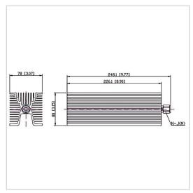
RF Solution offer a wide selection of Coaxial Fixed Termination (Dummy Load) for global customers. CT-200W-FA8022-NJ-3G is a Coaxial Fixed Termination (Dummy Load) in Frequency Range of DC $\sim$ 3.0 GHz. It is made of high quality materials under a high standard, the Connector Type of this product is N-M (J), VSWR Max is 1.25 and Impedance is 50  $\Omega$ . The component has a good working performance and stability, it is ideal for handling a Power of 200 W.
