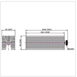
RF Solution offer a wide selection of Coaxial Fixed Termination (Dummy Load) for global customers. CT-200W-FA8022-DINK-4G is a Coaxial Fixed Termination (Dummy Load) in Frequency Range of DC~4.0 GHz. It is made of high quality materials under a high standard, the Connector Type of this product is DIN-F (K), VSWR Max is 1.30 and Impedance is 50  $\Omega$ . The component has a good working performance and stability, it is ideal for handling a Power of 200 W.
