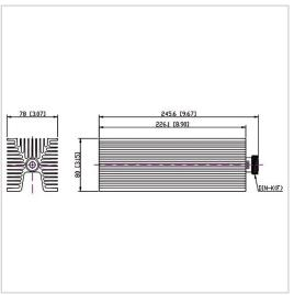
RF Solution offer a wide selection of Coaxial Fixed Termination (Dummy Load) for global customers. CT-200W-FA8022-DINK-3G is a Coaxial Fixed Termination (Dummy Load) in Frequency Range of DC $\sim$ 3.0 GHz. It is made of high quality materials under a high standard, the Connector Type of this product is DIN-F (K), VSWR Max is 1.25 and Impedance is 50  $\Omega$ . The component has a good working performance and stability, it is ideal for handling a Power of 200 W.
