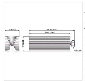
RF Solution offer a wide selection of Coaxial Fixed Termination (Dummy Load) for global customers. CT-200W-FA8022-DINJ-6G is a Coaxial Fixed Termination (Dummy Load) in Frequency Range of DC~6.0 GHz. It is made of high quality materials under a high standard, the Connector Type of this product is DIN-M (J), VSWR Max is 1.30 and Impedance is 50  $\Omega$ . The component has a good working performance and stability, it is ideal for handling a Power of 200 W.
