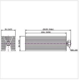
RF Solution offer a wide selection of Coaxial Fixed Termination (Dummy Load) for global customers. CT-200W-FA8022-DINJ-4G is a Coaxial Fixed Termination (Dummy Load) in Frequency Range of DC~4.0 GHz. It is made of high quality materials under a high standard, the Connector Type of this product is DIN-M (J), VSWR Max is 1.30 and Impedance is 50  $\Omega$ . The component has a good working performance and stability, it is ideal for handling a Power of 200 W.
