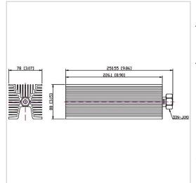
RF Solution offer a wide selection of Coaxial Fixed Termination (Dummy Load) for global customers. CT-200W-FA8022-DINJ-3G is a Coaxial Fixed Termination (Dummy Load) in Frequency Range of DC~3.0 GHz. It is made of high quality materials under a high standard, the Connector Type of this product is DIN-M (J), VSWR Max is 1.25 and Impedance is 50  $\Omega$ . The component has a good working performance and stability, it is ideal for handling a Power of 200 W.
