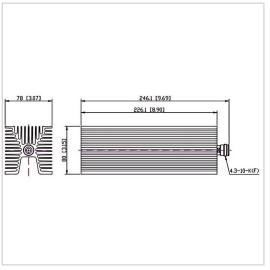
RF Solution offer a wide selection of Coaxial Fixed Termination (Dummy Load) for global customers. CT-200W-FA8022-4310K-6G is a Coaxial Fixed Termination (Dummy Load) in Frequency Range of DC $\sim$ 6.0 GHz. It is made of high quality materials under a high standard, the Connector Type of this product is 4.3-10-F (K), VSWR Max is 1.30 and Impedance is 50  $\Omega$ . The component has a good working performance and stability, it is ideal for handling a Power of 200 W.
