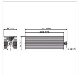
RF Solution offer a wide selection of Coaxial Fixed Termination (Dummy Load) for global customers. CT-200W-FA8022-4310K-4G is a Coaxial Fixed Termination (Dummy Load) in Frequency Range of DC~4.0 GHz. It is made of high quality materials under a high standard, the Connector Type of this product is 4.3-10-F (K), VSWR Max is 1.30 and Impedance is 50  $\Omega$ . The component has a good working performance and stability, it is ideal for handling a Power of 200 W.
