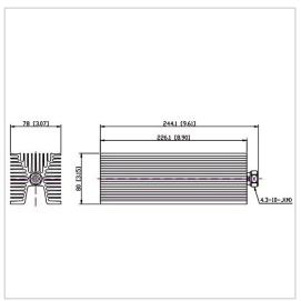
RF Solution offer a wide selection of Coaxial Fixed Termination (Dummy Load) for global customers. CT-200W-FA8022-4310J-6G is a Coaxial Fixed Termination (Dummy Load) in Frequency Range of DC~6.0 GHz. It is made of high quality materials under a high standard, the Connector Type of this product is 4.3-10-M (J), VSWR Max is 1.30 and Impedance is 50  $\Omega$ . The component has a good working performance and stability, it is ideal for handling a Power of 200 W.
