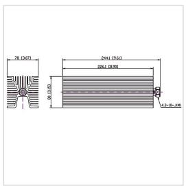
RF Solution offer a wide selection of Coaxial Fixed Termination (Dummy Load) for global customers. CT-200W-FA8022-4310J-4G is a Coaxial Fixed Termination (Dummy Load) in Frequency Range of DC~4.0 GHz. It is made of high quality materials under a high standard, the Connector Type of this product is 4.3-10-M (J), VSWR Max is 1.30 and Impedance is 50  $\Omega$ . The component has a good working performance and stability, it is ideal for handling a Power of 200 W.
