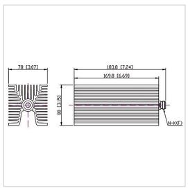
RF Solution offer a wide selection of Coaxial Fixed Termination (Dummy Load) for global customers. CT-150W-FA8017-NK-6G is a Coaxial Fixed Termination (Dummy Load) in Frequency Range of DC $\sim$ 6.0 GHz. It is made of high quality materials under a high standard, the Connector Type of this product is N-F (K), VSWR Max is 1.30 and Impedance is 50  $\Omega$ . The component has a good working performance and stability, it is ideal for handling a Power of 150 W.
