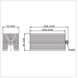
RF Solution offer a wide selection of Coaxial Fixed Termination (Dummy Load) for global customers. CT-150W-FA8017-NK-4G is Coaxial Fixed а Termination (Dummy Load) in Frequency Range of DC~4.0 GHz. It is made of high quality materials under a high standard, the Connector Type of this product is N-F (K), VSWR Max is 1.25 and Impedance is 50  $\Omega$ . The component has a good working performance and stability, it is ideal for handling a Power of 150 W.
