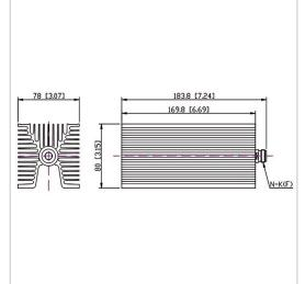
RF Solution offer a wide selection of Coaxial Fixed Termination (Dummy Load) for global customers. CT-150W-FA8017-NK-3G is a Coaxial Fixed Termination (Dummy Load) in Frequency Range of DC~3.0 GHz. It is made of high quality materials under a high standard, the Connector Type of this product is N-F (K), VSWR Max is 1.20 and Impedance is 50  $\Omega$ . The component has a good working performance and stability, it is ideal for handling a Power of 150 W.
