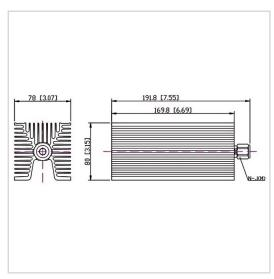
RF Solution offer a wide selection of Coaxial Fixed Termination (Dummy Load) for global customers. CT-150W-FA8017-NJ-3G is a Coaxial Fixed Termination (Dummy Load) in Frequency Range of DC $\sim$ 3.0 GHz. It is made of high quality materials under a high standard, the Connector Type of this product is N-M (J), VSWR Max is 1.20 and Impedance is 50  $\Omega$ . The component has a good working performance and stability, it is ideal for handling a Power of 150 W.
