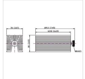
RF Solution offer a wide selection of Coaxial Fixed Termination (Dummy Load) for global customers. CT-150W-FA8017-DINK-6G is a Coaxial Fixed Termination (Dummy Load) in Frequency Range of DC~6.0 GHz. It is made of high quality materials under a high standard, the Connector Type of this product is DIN-F (K), VSWR Max is 1.30 and Impedance is 50  $\Omega$ . The component has a good working performance and stability, it is ideal for handling a Power of 150 W.
