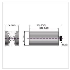
RF Solution offer a wide selection of Coaxial Fixed Termination (Dummy Load) for global customers. CT-150W-FA8017-DINK-4G is a Coaxial Fixed Termination (Dummy Load) in Frequency Range of DC~4.0 GHz. It is made of high quality materials under a high standard, the Connector Type of this product is DIN-F (K), VSWR Max is 1.30 and Impedance is 50  $\Omega$ . The component has a good working performance and stability, it is ideal for handling a Power of 150 W.
