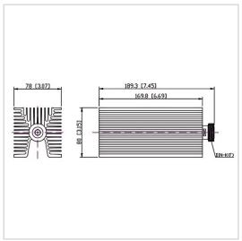
RF Solution offer a wide selection of Coaxial Fixed Termination (Dummy Load) for global customers. CT-150W-FA8017-DINK-3G is a Coaxial Fixed Termination (Dummy Load) in Frequency Range of DC $\sim$ 3.0 GHz. It is made of high quality materials under a high standard, the Connector Type of this product is DIN-F (K), VSWR Max is 1.25 and Impedance is 50  $\Omega$ . The component has a good working performance and stability, it is ideal for handling a Power of 150 W.
