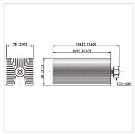
RF Solution offer a wide selection of Coaxial Fixed Termination (Dummy Load) for global customers. CT-150W-FA8017-DINJ-6G is a Coaxial Fixed Termination (Dummy Load) in Frequency Range of DC~6.0 GHz. It is made of high quality materials under a high standard, the Connector Type of this product is DIN-M (J), VSWR Max is 1.30 and Impedance is 50  $\Omega$ . The component has a good working performance and stability, it is ideal for handling a Power of 150 W.
