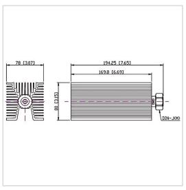
RF Solution offer a wide selection of Coaxial Fixed Termination (Dummy Load) for global customers. CT-150W-FA8017-DINJ-4G is a Coaxial Fixed Termination (Dummy Load) in Frequency Range of DC~4.0 GHz. It is made of high quality materials under a high standard, the Connector Type of this product is DIN-M (J), VSWR Max is 1.30 and Impedance is 50  $\Omega$ . The component has a good working performance and stability, it is ideal for handling a Power of 150 W.
