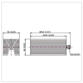
RF Solution offer a wide selection of Coaxial Fixed Termination (Dummy Load) for global customers. CT-150W-FA8017-4310K-3G is a Coaxial Fixed Termination (Dummy Load) in Frequency Range of DC $\sim$ 3.0 GHz. It is made of high quality materials under a high standard, the Connector Type of this product is 4.3-10-F (K), VSWR Max is 1.25 and Impedance is 50  $\Omega$ . The component has a good working performance and stability, it is ideal for handling a Power of 150 W.
