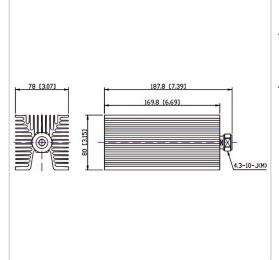
RF Solution offer a wide selection of Coaxial Fixed Termination (Dummy Load) for global customers. CT-150W-FA8017-4310J-6G is a Coaxial Fixed Termination (Dummy Load) in Frequency Range of DC~6.0 GHz. It is made of high quality materials under a high standard, the Connector Type of this product is 4.3-10-M (J), VSWR Max is 1.30 and Impedance is 50  $\Omega$ . The component has a good working performance and stability, it is ideal for handling a Power of 150 W.
