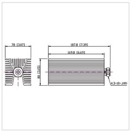
RF Solution offer a wide selection of Coaxial Fixed Termination (Dummy Load) for global customers. CT-150W-FA8017-4310J-3G is a Coaxial Fixed Termination (Dummy Load) in Frequency Range of DC~3.0 GHz. It is made of high quality materials under a high standard, the Connector Type of this product is 4.3-10-M (J), VSWR Max is 1.20 and Impedance is 50  $\Omega$ . The component has a good working performance and stability, it is ideal for handling a Power of 150 W.
