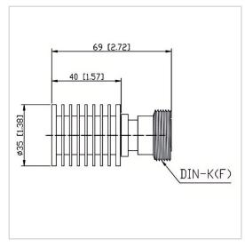
RF Solution offer a wide selection of Coaxial Low PIM Termination for global customers. CT-10W-RH3540-IP65-DINK-3G is а Coaxial Low PIM Termination in Frequency Range of DC~3.0 GHz. It is made of high quality materials under a high standard, the Connector Type of this product is DIN-F (K), VSWR Max is 1.20 and Impedance is 50  $\Omega$ . The component has a good working performance and stability, it is ideal for handling a Power of 10 W.
