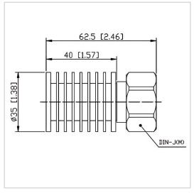
RF Solution offer a wide selection of Coaxial Low PIM Termination for global customers. CT-10W-RH3540-IP65-DINJ-3G is а Coaxial Low Termination in Frequency Range of DC~3.0 GHz. It is made of high quality materials under a high standard, the Connector Type of this product is DIN-M (J), VSWR Max is 1.20 and Impedance is 50  $\Omega$ . The component has a good working performance and stability, it is ideal for handling a Power of 10 W.
