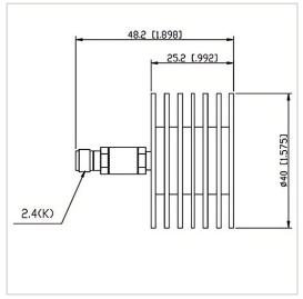
RF Solution offer a wide selection of Coaxial Fixed Termination (Dummy Load) for global customers. CT-10W-RA4025-2.4K-50G is a Coaxial Fixed Termination (Dummy Load) in Frequency Range of DC~50.0 GHz. It is made of high quality materials under a high standard, the Connector Type of this product is 2.4-F (K), VSWR Max is 1.40 and Impedance is 50  $\Omega$ . The component has a good working performance and stability, it is ideal for handling a Power of 10 W.
