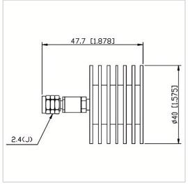
RF Solution offer a wide selection of Coaxial Fixed Termination (Dummy Load) for global customers. CT-10W-RA4025-2.4J-50G is a Coaxial Fixed Termination (Dummy Load) in Frequency Range of DC~50.0 GHz. It is made of high quality materials under a high standard, the Connector Type of this product is 2.4-M (J), VSWR Max is 1.40 and Impedance is 50  $\Omega$ . The component has a good working performance and stability, it is ideal for handling a Power of 10 W.
