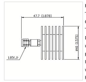
RF Solution offer a wide selection of Coaxial Fixed Termination (Dummy Load) for global customers. CT-10W-RA4025-1.85J-67G is a Coaxial Fixed Termination (Dummy Load) in Frequency Range of DC~67.0 GHz. It is made of high quality materials under a high standard, the Connector Type of this product is 1.85-M (J), VSWR Max is 1.40 and Impedance is 50  $\Omega$ . The component has a good working performance and stability, it is ideal for handling a Power of 10 W.
