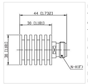
RF Solution offer a wide selection of Coaxial Fixed Termination (Dummy Load) for global customers. CT-10W-RA3030-NK-8G is a Coaxial Fixed Termination (Dummy Load) in Frequency Range of DC~8.0 GHz. It is made of high quality materials under a high standard, the Connector Type of this product is N-F (K), VSWR Max is 1.20 and Impedance is 50  $\Omega$ . The component has a good working performance and stability, it is ideal for handling a Power of 10 W.
