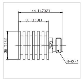
RF Solution offer a wide selection of Coaxial Fixed Termination (Dummy Load) for global customers. CT-10W-RA3030-NK-6G is a Coaxial Fixed Termination (Dummy Load) in Frequency Range of DC~6.0 GHz. It is made of high quality materials under a high standard, the Connector Type of this product is N-F (K), VSWR Max is 1.20 and Impedance is 50  $\Omega$ . The component has a good working performance and stability, it is ideal for handling a Power of 10 W.
