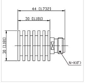
RF Solution offer a wide selection of Coaxial Fixed Termination (Dummy Load) for global customers. CT-10W-RA3030-NK-3G is a Coaxial Fixed Termination (Dummy Load) in Frequency Range of DC $\sim$ 3.0 GHz. It is made of high quality materials under a high standard, the Connector Type of this product is N-F (K), VSWR Max is 1.20 and Impedance is 50  $\Omega$ . The component has a good working performance and stability, it is ideal for handling a Power of 10 W.
