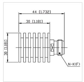
RF Solution offer a wide selection of Coaxial Fixed Termination (Dummy Load) for global customers. CT-10W-RA3030-NK-18G is a Coaxial Fixed Termination (Dummy Load) in Frequency Range of DC~18.0 GHz. It is made of high quality materials under a high standard, the Connector Type of this product is N-F (K), VSWR Max is 1.25 and Impedance is 50  $\Omega$ . The component has a good working performance and stability, it is ideal for handling a Power of 10 W.
