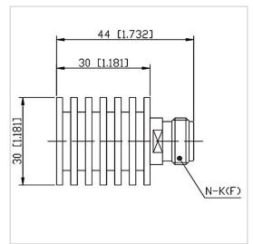
RF Solution offer a wide selection of Coaxial Fixed Termination (Dummy Load) for global customers. CT-10W-RA3030-NK-12.4G is a Coaxial Fixed Termination (Dummy Load) in Frequency Range of DC~12.4 GHz. It is made of high quality materials under a high standard, the Connector Type of this product is N-F (K), VSWR Max is 1.25 and Impedance is 50  $\Omega$ . The component has a good working performance and stability, it is ideal for handling a Power of 10 W.
