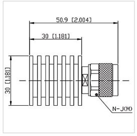
RF Solution offer a wide selection of Coaxial Fixed Termination (Dummy Load) for global customers. CT-10W-RA3030-NJ-8G is a Coaxial Fixed Termination (Dummy Load) in Frequency Range of DC~8.0 GHz. It is made of high quality materials under a high standard, the Connector Type of this product is N-M (J), VSWR Max is 1.20 and Impedance is 50  $\Omega$ . The component has a good working performance and stability, it is ideal for handling a Power of 10 W.
