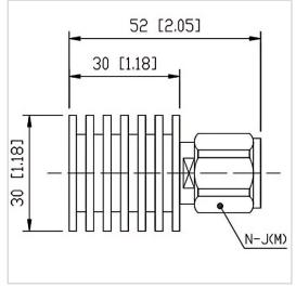
RF Solution offer a wide selection of Coaxial Fixed Termination (Dummy Load) for global customers. CT-10W-RA3030-NJ-6G is a Coaxial Fixed Termination (Dummy Load) in Frequency Range of DC~6.0 GHz. It is made of high quality materials under a high standard, the Connector Type of this product is N-M (J), VSWR Max is 1.20 and Impedance is 50  $\Omega$ . The component has a good working performance and stability, it is ideal for handling a Power of 10 W.
