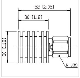
RF Solution offer a wide selection of Coaxial Fixed Termination (Dummy Load) for global customers. CT-10W-RA3030-NJ-3G is a Coaxial Fixed Termination (Dummy Load) in Frequency Range of DC~3.0 GHz. It is made of high quality materials under a high standard, the Connector Type of this product is N-M (J), VSWR Max is 1.20 and Impedance is 50  $\Omega$ . The component has a good working performance and stability, it is ideal for handling a Power of 10 W.
