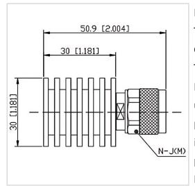
RF Solution offer a wide selection of Coaxial Fixed Termination (Dummy Load) for global customers. CT-10W-RA3030-NJ-18G is a Coaxial Fixed Termination (Dummy Load) in Frequency Range of DC~18.0 GHz. It is made of high quality materials under a high standard, the Connector Type of this product is N-M (J), VSWR Max is 1.30 and Impedance is 50  $\Omega$ . The component has a good working performance and stability, it is ideal for handling a Power of 10 W.
