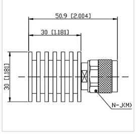
RF Solution offer a wide selection of Coaxial Fixed Termination (Dummy Load) for global customers. CT-10W-RA3030-NJ-12.4G is a Coaxial Fixed Termination (Dummy Load) in Frequency Range of DC~12.4 GHz. It is made of high quality materials under a high standard, the Connector Type of this product is N-M (J), VSWR Max is 1.25 and Impedance is 50  $\Omega$ . The component has a good working performance and stability, it is ideal for handling a Power of 10 W.
