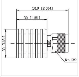
RF Solution offer a wide selection of Coaxial Fixed Termination (Dummy Load) for global customers. CT-10W-RA3030-NJ-10G is a Coaxial Fixed Termination (Dummy Load) in Frequency Range of DC~10.0 GHz. It is made of high quality materials under a high standard, the Connector Type of this product is N-M (J), VSWR Max is 1.25 and Impedance is 50  $\Omega$ . The component has a good working performance and stability, it is ideal for handling a Power of 10 W.
