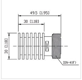
RF Solution offer a wide selection of Coaxial Fixed Termination (Dummy Load) for global customers. CT-10W-RA3030-DINK-6G is Coaxial Termination (Dummy Load) in Frequency Range of DC~6.0 GHz. It is made of high quality materials under a high standard, the Connector Type of this product is DIN-F (K), VSWR Max is 1.30 and Impedance is 50  $\Omega$ . The component has a good working performance and stability, it is ideal for handling a Power of 10 W.
